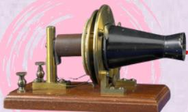
Alexander Graham Bell is credited with inventing the first working telephone. The device functions by turning sound waves into electrical signals that travel through wires, and then converting them back into sound at the other end.
